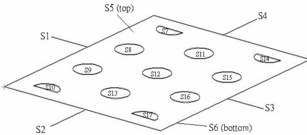
Figure 1(b). The geometry of plate fin in staggered arrangement.
