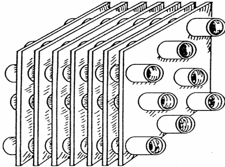
Figure 1(a). A typical plate finned-tube heat exchanger.
